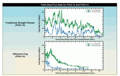
The US Navy research of 1994 compared 3D (offensive) fog against straight streams using the short burst and pause cycle
