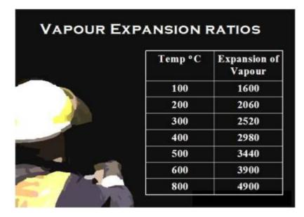
It can bee seen above that water vapour expansion is greater at higher temperatures. In a room fire the expansion ratio at 100°C Is known to be around 1600-1. However, as temperatures increase in the higher regions of the room the expansion of water vapour increases substantially and near the ceiling the expansion may be seen to be around 4000 or 5000-1
