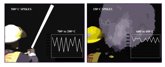
In these computer-simulated images from real fire data, the effect of high temperature evaporation at the ceiling using a flowrate of 360 lpm can be seen in the 500°C spikes (left) from a straight stream when compared to the less severe 150°C spikes from the 3D water-fog pattern (right)
