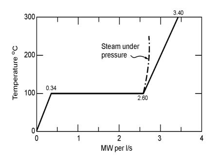
As water reaches it's boiling point under atmospheric conditions it offers its greatest cooling power during the transition from liquid into its vapour state. As this transition takes place 2.3MJ of heat is absorbed.
