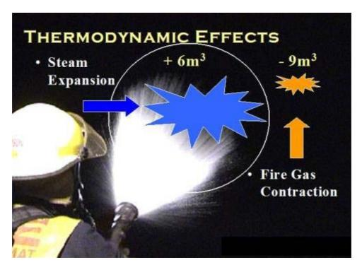
An example of thermodynamic effects where the expanding water vapour is countered by fire gas contraction
