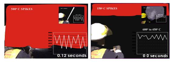
Further effects of high temperature vapour expansion where  $500^{\circ}$ C spikes and 4000-1 vapour expansions force the smoke and thermal layers down into the lower regions of the room. The less severe  $150^{\circ}$ C spikes from the 3D fog pattern enable the smoke and thermal layers to rise as the contraction of the cooling gases counters the expansion of vapour at 2700-1
